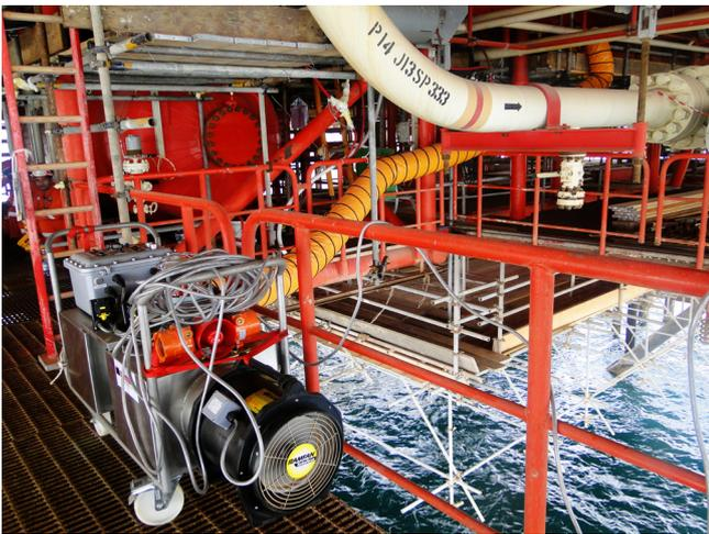
Figure 4. Fully customised Hot-Hed Habitat utilised on offshore platform.
